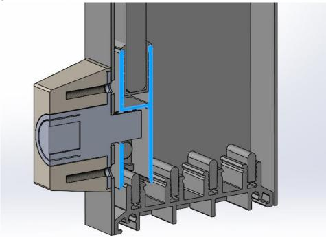
d. When the lock is mounted too low, it becomes more difficult to tighten the lower Allen screw.
