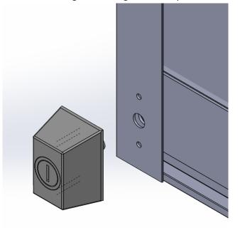
9. Mount the hole from the inside with the two m4 screws. Tighten it with an Allen key.
