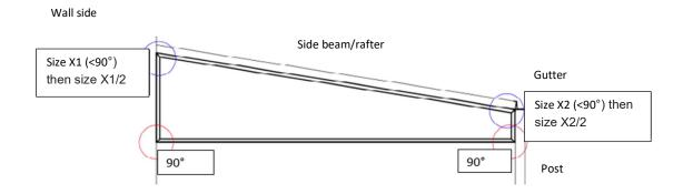
Now saw the polycarbonate sheet to size so that it falls into the F profiles at least 25 mm all around. Blow or vacuum all chambers after cutting.
