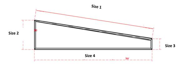
Now determine the inclination of the ends of Measure 1 and the upper corners of Measure 2 and 3. The ends of length 4 and the lower corners of Measure 2 and Measure 3 should have an angle of 45° (by default).
