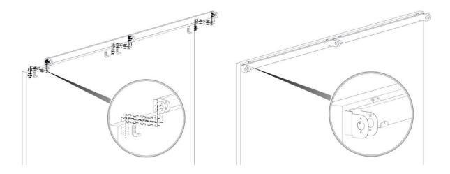
4. Fasten and tighten the wall mounting bracket bolts
