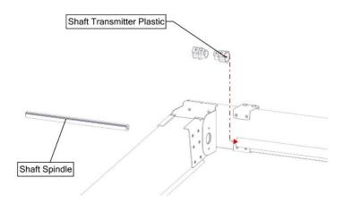
**6**. Place a shaft spindle through the rail and insert the shaft transmitter plastic on the spindle to connect to the other spindle.
